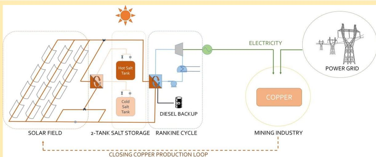
**Figure 3: Schematic description of the proposed integration of a CSP plant into the mining industry**
