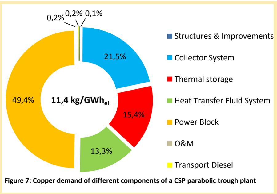
Based on this assessment a specific copper demand for solar energy generation with a parabolic trough plant of 11 kg/GWh<sub>el</sub> was calculated.
