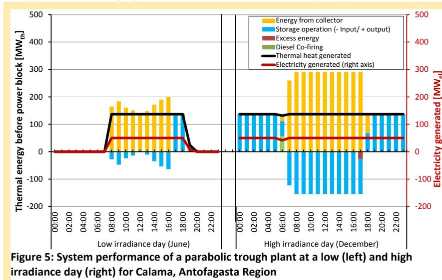
**Figure 5: System performance of a parabolic trough plant at a low (left) and high irradiance day (right) for Calama, Antofagasta Region**
